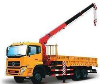
Truck Mounted Crane
